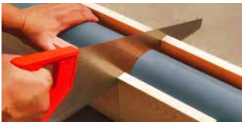
Figure 1 Pipe cutting with a hand-saw
